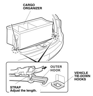
4. Adjust the length of the straps as needed to secure the organizer to the vehicle tie-down hooks.
