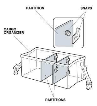
3. Place the organizer in the cargo area of the vehicle, and attach the outer hooks on the organizer to the vehicle tie-down hooks.
