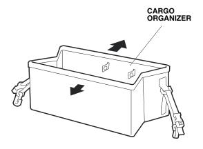
2. Attach the two partitions to the cargo organizer by connecting the inner snaps.
